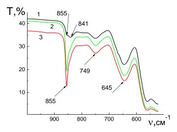
Figure 1: Alloyed germanium spectra (the maximum values of phonon absorption bands with indication of the corresponding wave numbers are shown with arrows)
